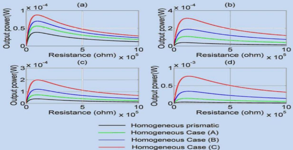
Variation of output power with external load resistance of homogeneous prismatic beam ( $c_b=0.0$ ,  $c_h=0.0$ ) and homogeneous nonprismatic beam for (a)  $c_b=0.1$ ,  $c_h=0.1$  (b)  $c_b=0.1$ ,  $c_h=0.3$  (c)  $c_b=0.3$ ,  $c_h=0.1$  and (d)  $c_b=0.3$ ,  $c_h=0.3$ .
